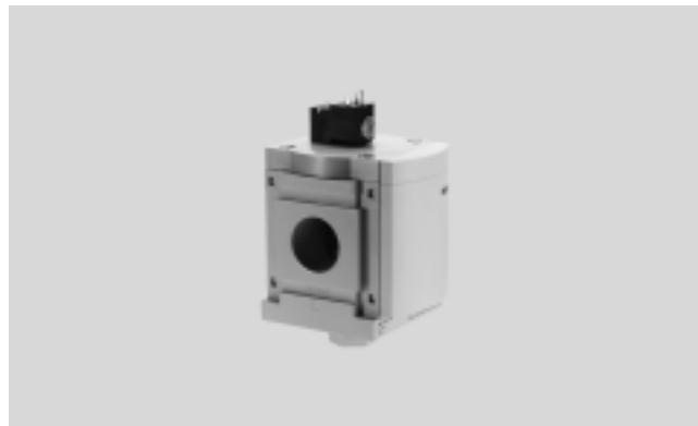
The duration of the pressure build-up is adjusted using the restrictor attached to the valve cap. The output pressure  $p_2$  rises slowly in accordance with the restrictor setting. Only the air flow from the restrictor is available when the solenoid valve is not actuated. The main seat is only opened by energising the solenoid valve.
