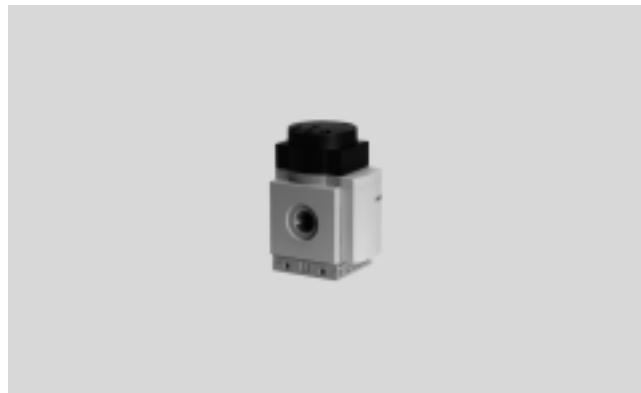
The duration of the pressure build-up is adjusted using the restrictor attached to the valve cap. The output pressure  $p_2$  rises slowly in accordance with the restrictor setting. The main seat opens when the switch-through pressure is reached.
